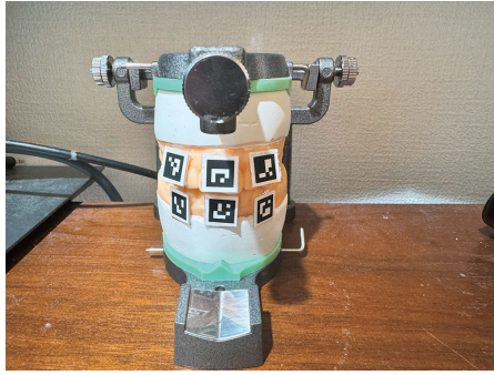
Figure 3: Marker Placement on Experimental Articulator
