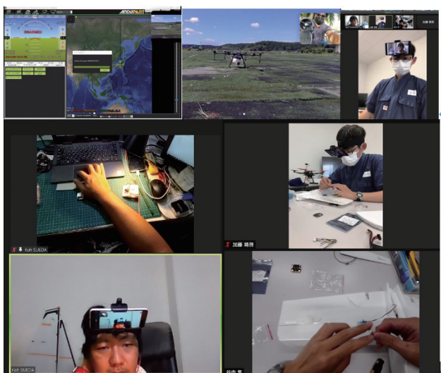
Figure 2: Remote OSUAV development workshop utilizing a simple collaboration environment where participants can see each other's hands, gaze, work environment, and screen through a smartphone mounted on a headgear.
