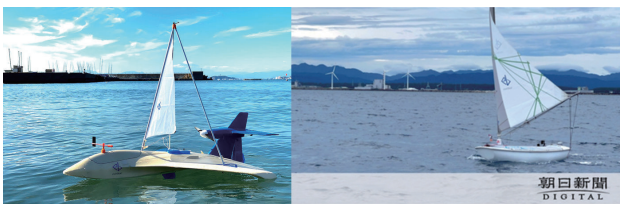
Figure6: FlyingSailboat developed using Ardupilot (left) and a sailing drone based on a Hansa Class1 sailboat (right).
