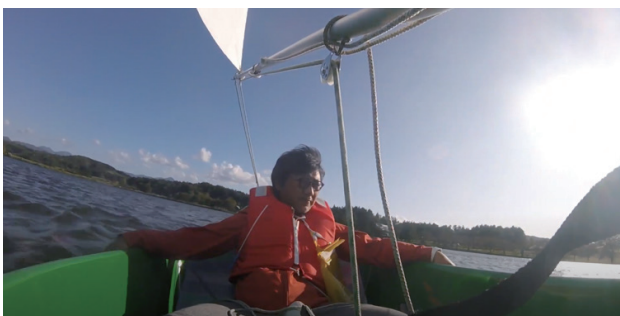
Figure8: OSUAV-applied Computer Aided Sailing experiment where the sailboat can sail autonomously and complement some of the sailor's operations.
