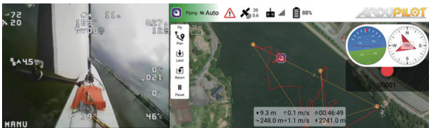
Figure7: Aiming at Computer Aided Sailing and applying OSUAV to develop a sailboat that assists the sailor. Equipped with automatic/semi-automatic sailing and automatic return functions
