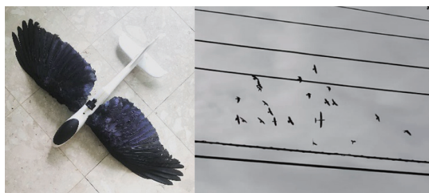
Figure 4: Prototype of a crow-shaped fixed-wing drone and a crow-guided test
