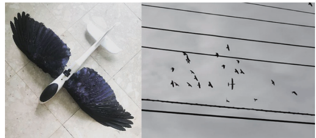
Figure 4: Prototype of a crow-shaped fixed-wing drone and a crow-guided test
